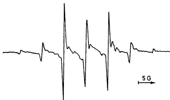
FIGURE 6 E.s.r. spectrum of the radical Bu_3SnOCMeCMeO^{\bullet} (IX) \rightleftharpoons (X) ( R = Bu_3Sn ) [ a(6H) 7.2 G], with an alternating linewidth effect, from the photolysis of a mixture of hexabutylditin, di- t -butyl peroxide, and biacetyl in toluene at -1 °C
