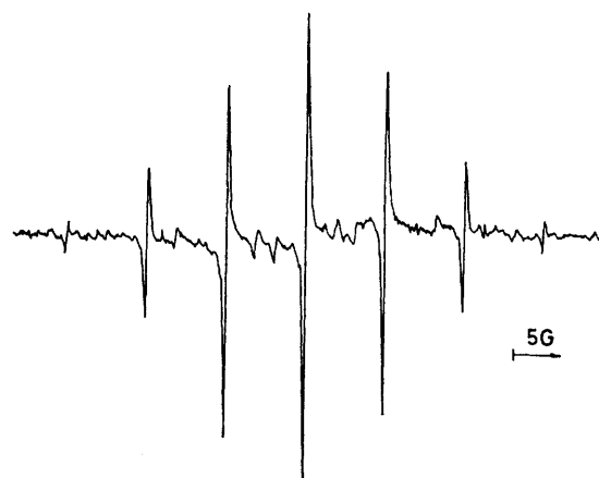
FIGURE 5 E.s.r. spectrum of the radical \text{Bu}_3\text{SnOCMeCMeO}\cdot (XVII) \rightleftharpoons (XVIII) [ a(6\text{H}) 8.5 G] from the photolysis of di- t -butyl peroxide in the presence of \text{Bu}_3\text{SnOCHMeCMeO} in cyclopropane at -109^\circ
